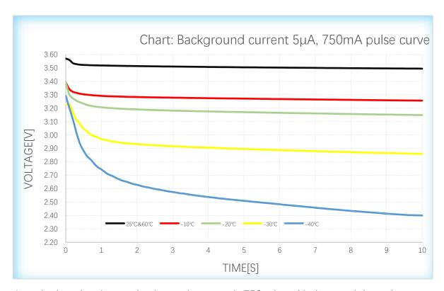
In a single pulse duty cycle, the peak current is 750mA and below, and the pulse capacity is 7.5AS/2.08mAh and below. You can refer to this graph for voltage design.
