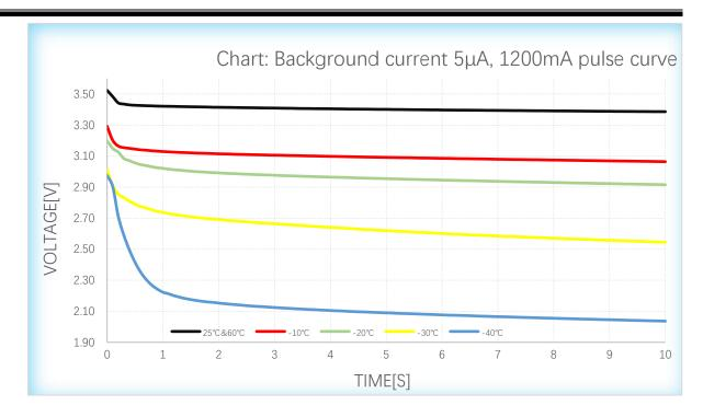
In a single pulse duty cycle, the peak current is 12600mA and below, and the pulse capacity is 12AS/3.3316mAh and below. You can refer to this graph for voltage design.
