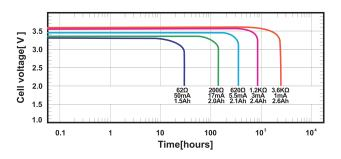
Typical Discharge Profiles at +23±2°C
