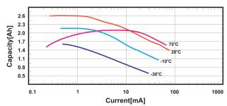
Capacity versus Current at various temperatures [ 2.0V cut-off ]
