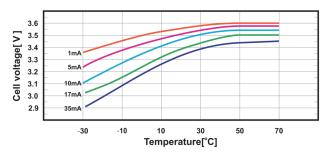
Voltage Plateau versus Current and Temperature
