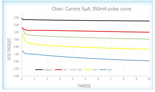
In a single pulse duty cycle, the peak current is 350mA and below, and the pulse capacity is 3.5AS/0.97mAh and below. You can refer to this graph for voltage design.
