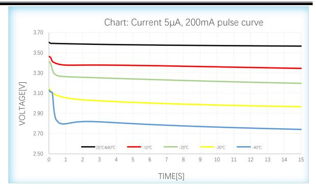
In a single pulse duty cycle, the peak current is 200mA and below, and the pulse capacity is 3.0AS/0.83mAh and below. You can refer to this graph for voltage design.
