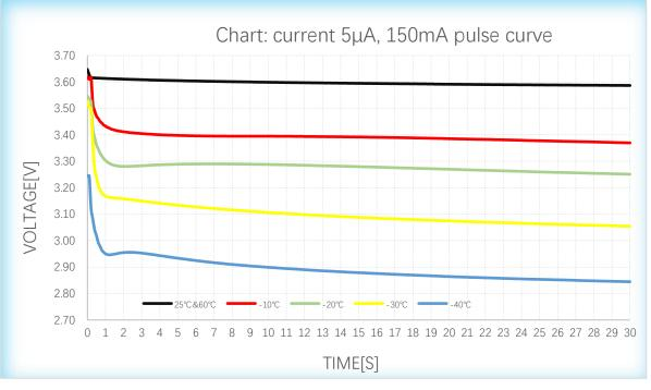
In a single pulse duty cycle, the peak current is 150mA and below, and the pulse capacity is 4.5AS/1.25mAh and below. You can refer to this graph for voltage design.
