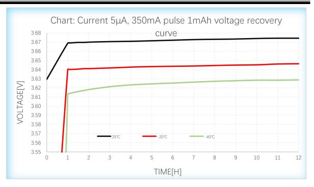
After a single pulse, before the next pulse arrives, when it is converted to a static background current of  $5\mu$ A, the voltage recovery of the battery pack within 12 hours. The pulse current is 350mA and below, the capacity is 1mAh and below, please refer to the voltage design of this graph
