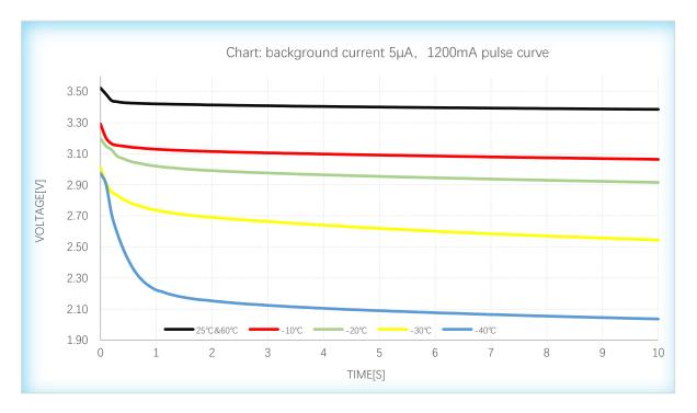
In a single pulse duty cycle, the peak current is 1200mA and below, and the pulse capacity is 12AS/3.331.66mAh and below. You can refer to this graph for voltage
