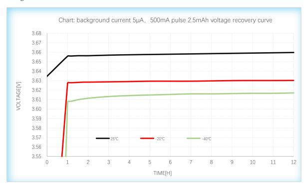
After a single pulse, before the next pulse arrives, when it is converted to a static background current of 5µA, the voltage recovery of the battery pack within 12 hours. The pulse current is 500mA and below, the capacity is 2.5mAh and below, please refer to the voltage design of this graph.
