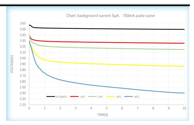
In a single pulse duty cycle, the peak current is 750mA and below, and the pulse capacity is 7.5AS/2.08mAh and below. You can refer to this graph for voltage design.
