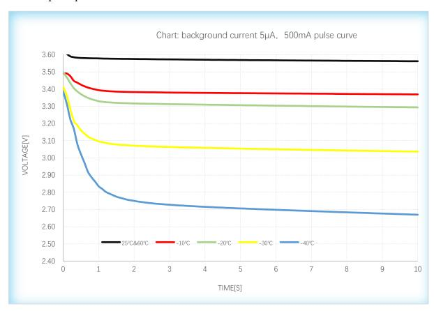
In a single pulse duty cycle, the peak current is 500mA and below, and the pulse capacity is 5AS/1.39mAh and below. You can refer to this graph for voltage design.
