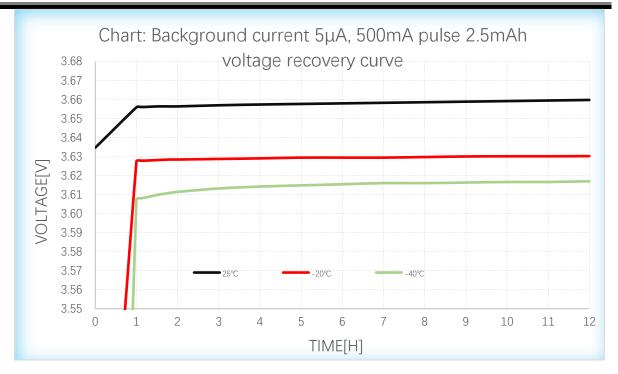
After a single pulse, before the arrival of the next pulse, when it is converted to a static background current of 5µA, the voltage recovery of the battery pack within 12 hours. The pulse current is 500mA and below, and the capacity is 2.5mAh and below. You can refer to this graph for voltage design.
