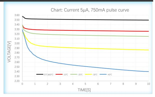
In a single pulse duty cycle, the peak current is 750mA and below, and the pulse
