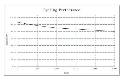
Remark: Charge:50mA to 4.1V Discharge 125mA to 2.5V @RT
